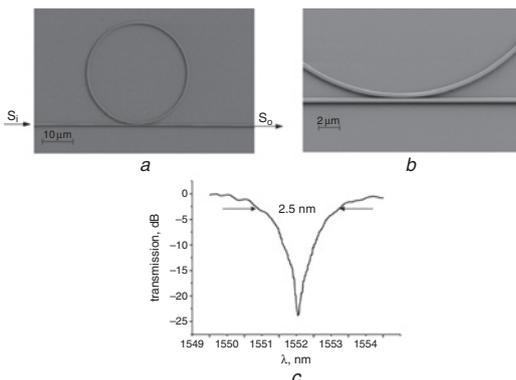
**Fig. 1** SEM photo of fabricated single coupled silicon microring resonator (cross-section of silicon waveguide 450  $\times$  250 nm<sup>2</sup>); zoom-in view of coupling region; measured transmission spectrum of silicon ring resonator
