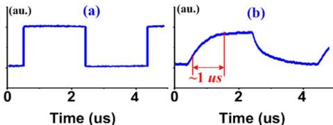
Fig. 6. (a) Waveform of the original baseband data. (b) Waveform of the down-converted data.
