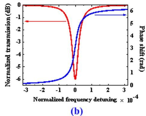
Fig. 1. (a) Basic structure of a single microring resonator. (b) Corresponding transmission spectrum and phase shift curve.
