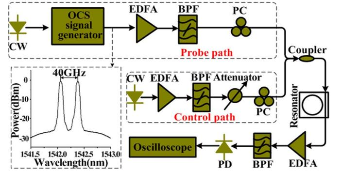
Fig. 3. Experimental setup for the proposed photonic RF phase shifter. CW: continuous wave; EDFA: erbium-doped fiber amplifier; BPF: bandpass filter; PC: polarization controller; and PD: photo-detector.
