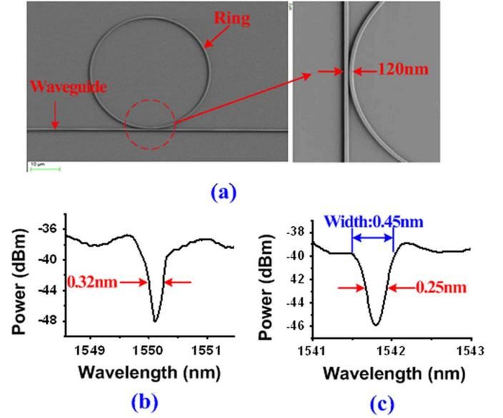
Fig. 2. (a) SEM photo of the microring resonator. (b) Spectrum of the device at 1550.1 nm. (c) Spectrum of the device at 1541.8 nm.
