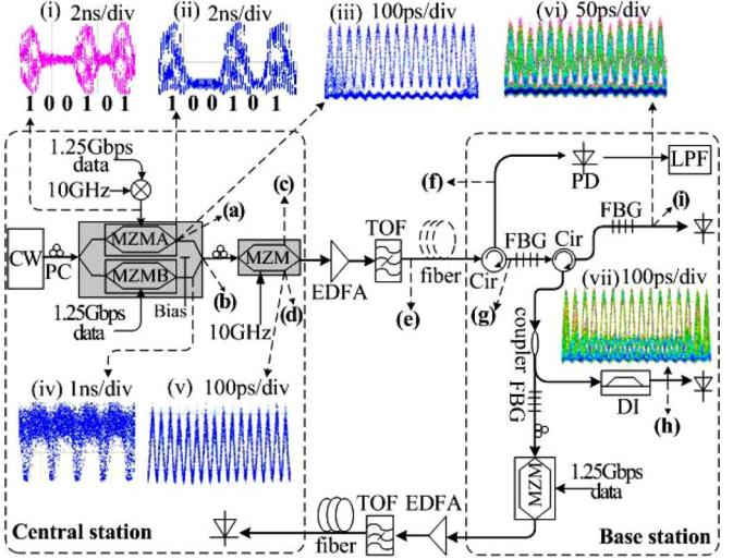
Fig. 2. Experimental setup of the proposed bidirectional RoF system. (i) The waveform of electrical SCM signal; (ii) the waveform of the optical SCM signal; (iii) the eye diagram of optical SCM signal; (iv) the eye diagram of DPSK signal; (v) the eye diagram optical MW signal; (vi) the eye diagram of optical MMW signal (back-to-back); (vii) the eye diagram of optical MW after MZDI (back-to-back). (a)–(i) correspond to the optical spectra shown in the Fig. 3.
