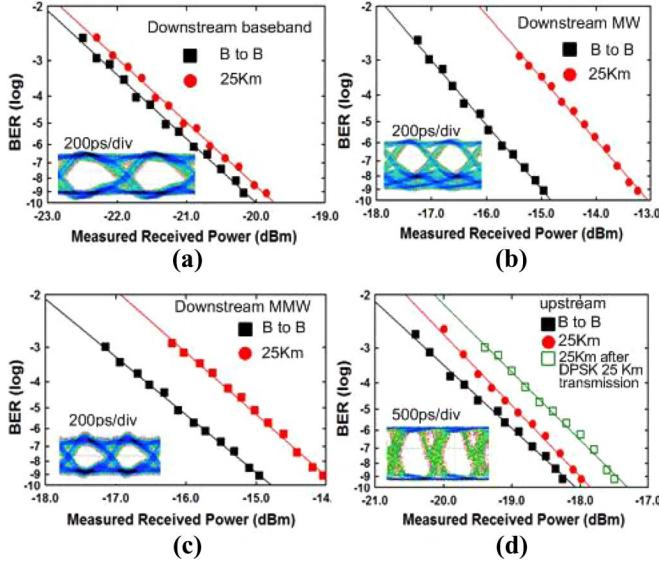
Fig. 4. BER curves and electrical eye diagrams. (a) Downstream baseband signal. (b) Downstream MW signal. (c) Downstream MMW signal. (d) Upstream remodulation signal.
