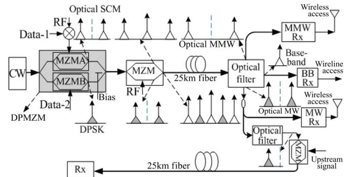
Fig. 1. Schematic diagram of the proposed bidirectional RoF system.
