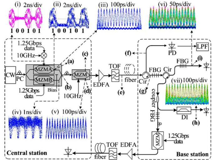
Fig. 2. Experimental setup of the proposed bidirectional RoF system. (i) The waveform of electrical SCM signal; (ii) the waveform of the optical SCM signal; (iii) the eye diagram of optical SCM signal; (iv) the eye diagram of DPSK signal; (v) the eye diagram of optical MW signal; (vi) the eye diagram of optical MMW signal (back-to-back); (vii) the eye diagram of optical MW after MZDI (back-to-back). (a)–(i) correspond to the optical spectra shown in the Fig. 3.
