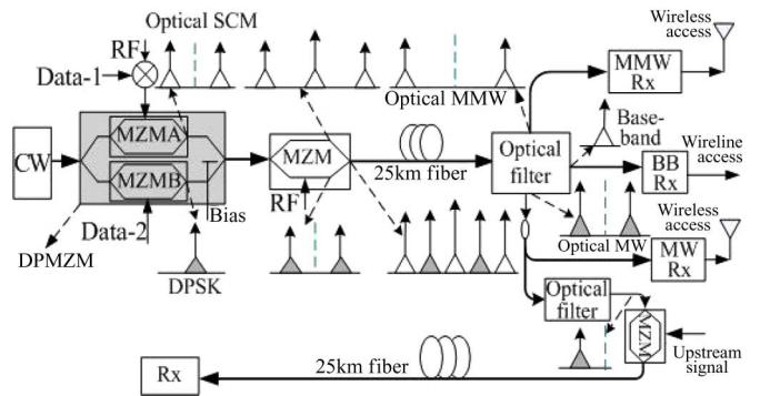
Fig. 1. Schematic diagram of the proposed bidirectional RoF system.
