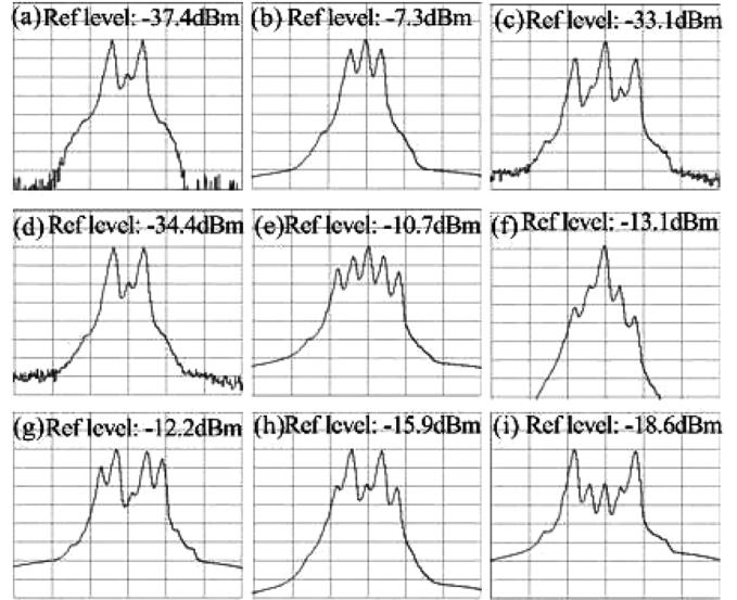
Fig. 3. Optical spectra taken at different positions as indicated in Fig. 2. Spectrum resolution: 0.07 nm; Start wavelength: 1548.86 nm; Stop wavelength: 1550.86 nm; X-axis scale: 0.2 nm/div, Y-axis scale: 5 dB/div. (a) Carrier-suppressed optical SCM signal; (b) DPMZM output signals; (c) baseband and MMW signals; (d) MW signal; (e) amplified multiband signals; (f) separated baseband signal; (g) passing signal from the first FBG; (h) separated MW signal; (i) separated MMW signal.
