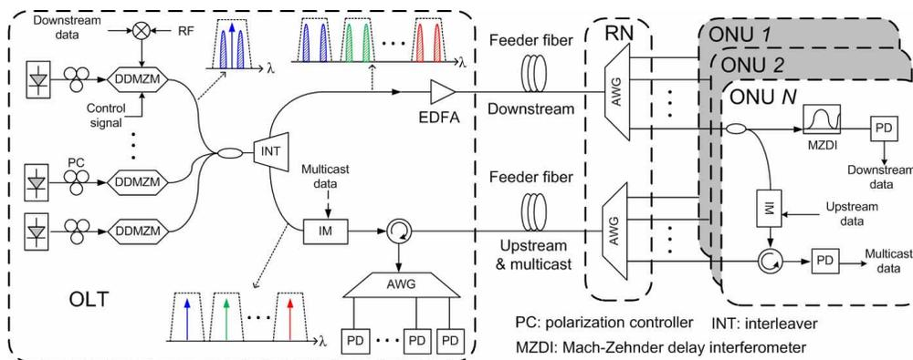
Fig. 1. Architecture of the proposed WDM PON with multicasting capability.
