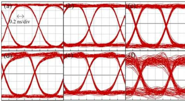
**Fig. 7.** The electrical eye-diagrams of the baseband signals down-converted from (a) 10-GHz, (b) 30-GHz, and (c) 50-GHz PSK-RF-signals without transmission; (d)–(f) are the corresponding eye-diagrams after the 25-km transmission.
