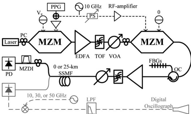
Fig. 3. Experimental setup. Note that the gray part is for the simulation. TOF: tunable optical filter; VOA: variable optical attenuator; OC: optical circulator; PC: polarization controller; LPF: low-pass filter.
