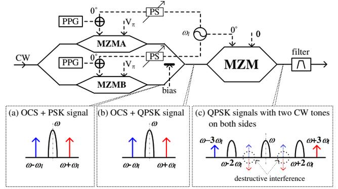
**Fig. 2.** Principle of the generation of QPSK modulated radio frequency signals: (a) simultaneous OCS modulation and PSK modulation by the MZMA, (b) QPSK signal and two CW tones, (c) three QPSK signals with two CW tones on both sides.
