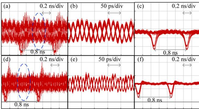
**Fig. 5.** Simulation results for the generation of 30-GHz and 50-GHz PSK-RF-signal: (a) electrical eye-diagram of the 30-GHz PSK-RF-signal; (b) magnified picture of the RF carrier in the blue circle in (a); (c) the PSK envelope; and (d)–(f) are the corresponding results for the 50-GHz case.
