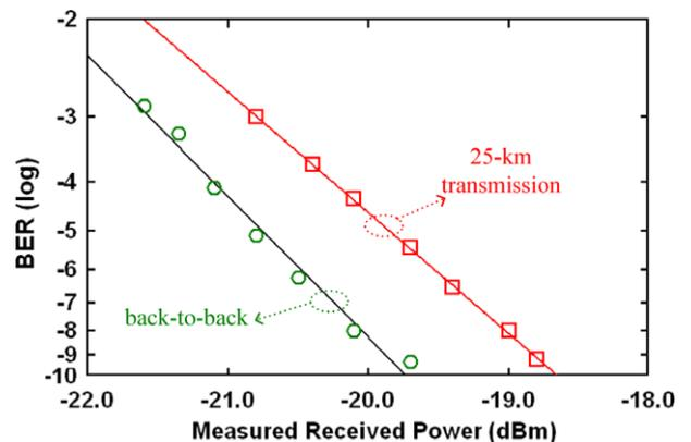
**Fig. 6.** Bit-error-rate performance of baseband PSK signal with and without 25-km transmission.
