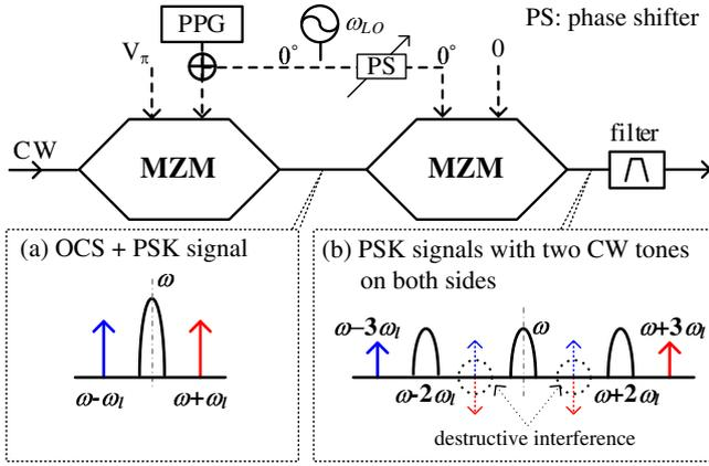
**Fig. 1.** Principle of the generation of PSK modulated radio frequency signals: (a) simultaneous optical carrier suppressed modulation and PSK modulation by the MZM, (b) three PSK signals with two CW tones on both sides.
