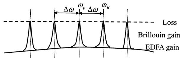
Fig. 4. Gain profile of each roundup trip for the self-seeded BEFL. EDFA, erbium-doped fiber amplifier.
