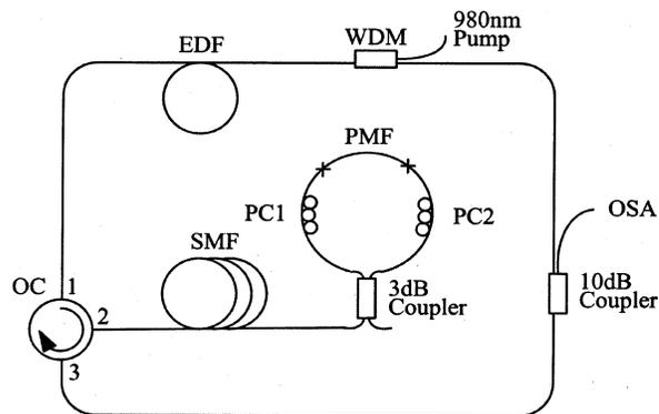
Fig. 1. Schematic of the self-seeded multiwavelength BEFL: WDM, 980/1550 wavelength-division multiplexer; OSA, optical spectrum analyzer; OC, optical circulator.
