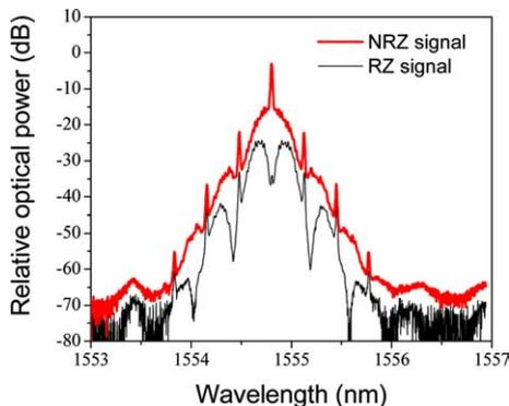
Fig. 4. Measured optical spectra. BW: 0.01 nm.
