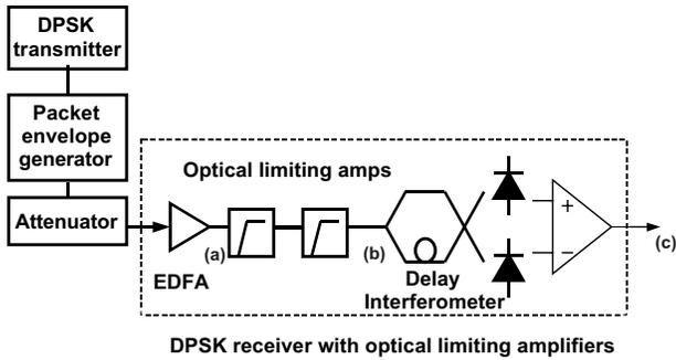
Fig. 2. Simplified schematic of the experimental setup.
