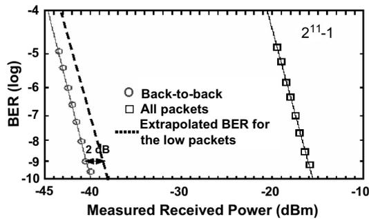
Fig. 4. BER measurement of back-to-back continuous data stream and packet reception with 25-dB DR. Dashed line is the derived BER curve for the low-level packet, showing 2-dB penalty compared to back-to-back continuous data measurement.
