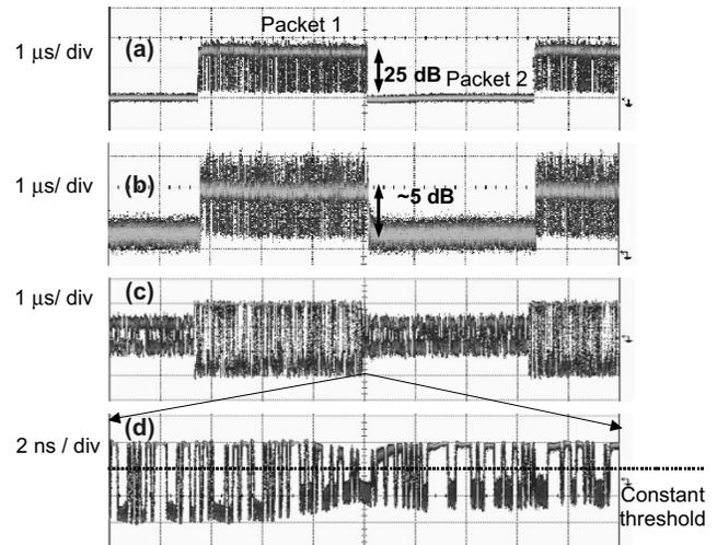
Fig. 3. (a) Optical DPSK signal after the preamplifier, (b) optical signal after the LOAs, (c) electric signal after balance detection and amplification, and (d) zoom-in picture of the electric signal.
