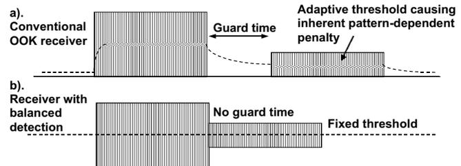
Fig. 1. Threshold in (a) conventional OOK receivers, and (b) balanced-detection receivers.
