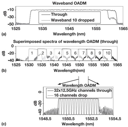
Fig. 2. (a) Waveband OADM transmission characteristic. (b) Wavelength OADM transmission characteristic for all channels through. Spectra are superimposed to show that the wavelength OADM can be shifted to any waveband. (c) Transmission characteristic of the wavelength OADM (set in Waveband 7) at through and odd-channel drop conditions, respectively.
