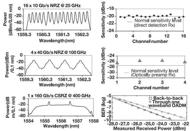
Fig. 3. Optical spectra of 10-, 40-, and 160-Gb/s signals of  $2^{31} - 1$  and their corresponding receiver sensitivity measurements through the OADM node.
