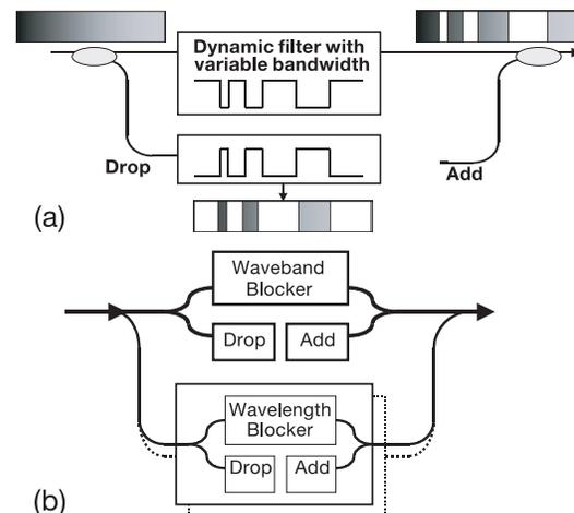
Fig. 1. (a) Illustration of the variable-bandwidth OADM at the wavelength level. (b) Hierarchical OADM consisting of wavelength and waveband levels to reduce the control complexity.
