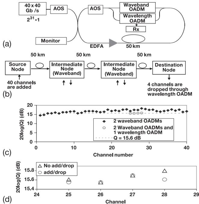
Fig. 4. (a) Recirculating loop setup to demonstrate multihop waveband and wavelength add-drop. AOS: acoustooptic switch. (b) Corresponding network scenario. (c)  $Q$  measurements. (d) Comparison of all through traffic with add-drop of neighboring waveband signals.
