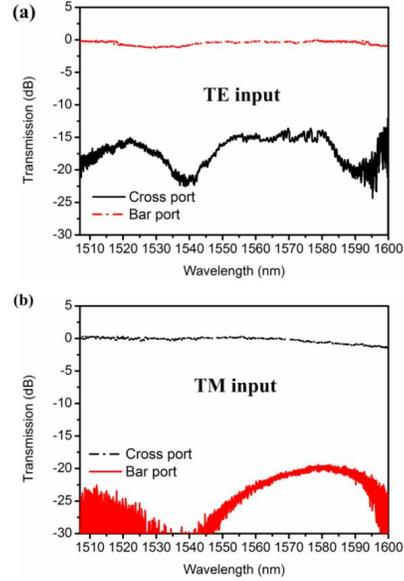
Fig. 4: Measured transmission responses at the Bar and Cross ports for (a) TE-polarized and (b) TM-polarized inputs.
