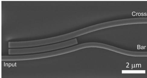
Fig. 3: Scanning electron microscope (SEM) photo of the fabricated PBS based on a bridged bent directional coupler.
