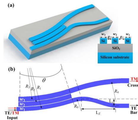
Fig. 1 Schematic configuration of the proposed silicon PBS.
