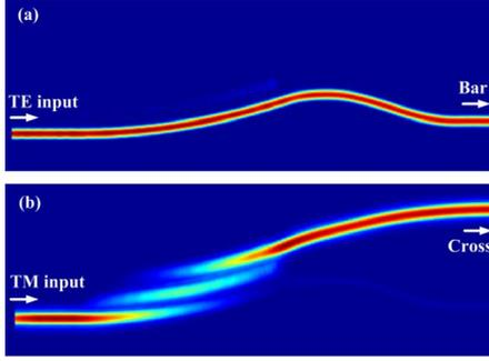
Fig. 2: (a)-(b) Simulated power distributions in the PBS for the TE- and TM-polarized inputs, respectively.
