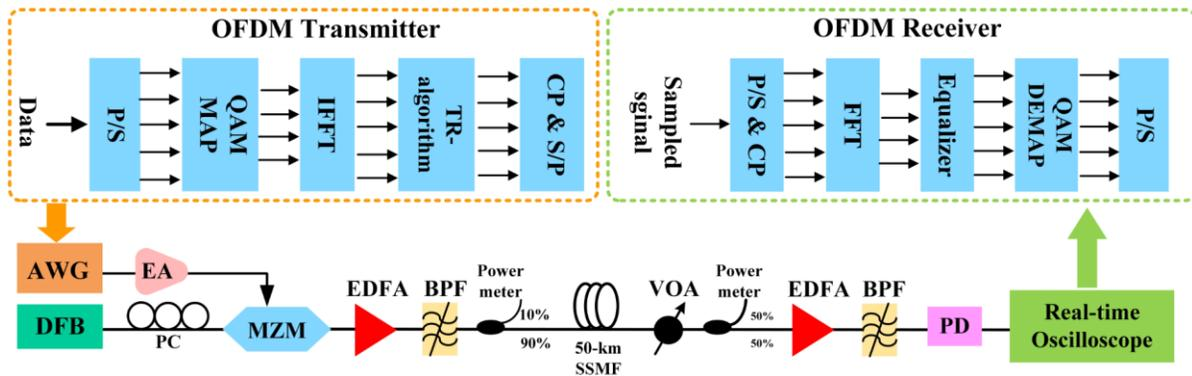
Fig. 2. Block diagram of the experimental setup for an intensity-modulated direct-detection (IM-DD) optical OFDM system with the proposed PAPR reduced method. EA: electrical amplifier, PC: polarization controller, VOA: variable optical attenuator, QAM: quadrature amplitude modulation, P/S: parallel to serial conversion, S/P: serial to parallel conversion.
