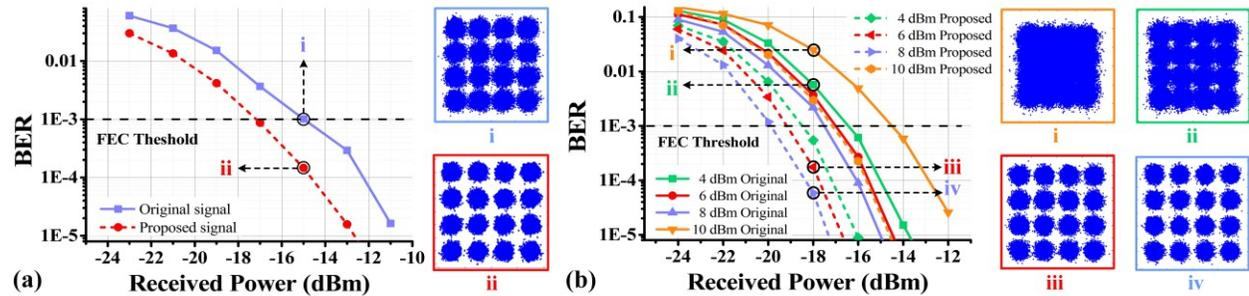
Fig. 3. BER curves of the original OFDM signal and the proposed TR-OFDM signal after 50-km SSMF transmission for (a) a launch power of  $\sim 2.5$  dBm. (b) launch powers of 4 dBm, 6 dBm, 8 dBm, and 10 dBm.
