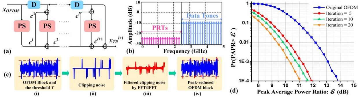
Fig. 1. (a) Algorithm of generating TR-OFDM signal. D: step delay, PS: peak search. (b) PRT allocations. (c) Waveforms in different steps of the proposed algorithm. (i) and (ii) Clipping step. (iii) Filtering step. (iv) Peak cancellation step, in which present the OFDM block (red) and the PAPR-reduced block (blue). (d) PAPR CCDFs for the original OFDM signal and the proposed TR-OFDM signal for various iterations.
