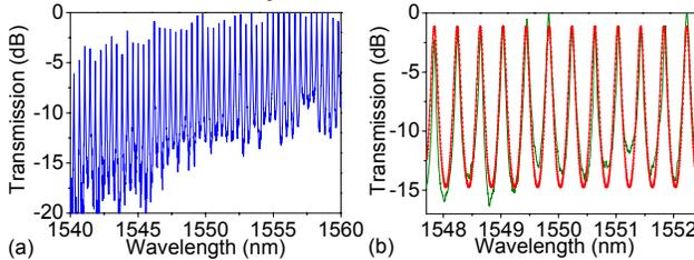
Fig. 3. (a) Measured transmission spectrum of the comb filter. (b) Measured (green-solid curve) and fitted (red-dot curve) transmission spectra in the wavelength range from 1547.5 nm to 1552.5 nm.
