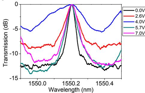
Fig. 5. Measured transmission spectra with various bandwidths at the same central wavelength by applying 0–7 V DC voltages.
