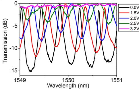
Fig. 4. Measured transmission spectra of the comb filter by applying 0–3.2 V DC voltages.
