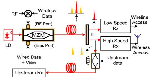
Fig. 1. Schematic diagram of the proposed RoF system with independent wired and wireless data driven by a single-drive MZM.
