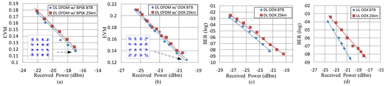
Fig. 4. EVM values and BER performances. (a) DL wireless OFDM signal with wired BPSK signal. (b) DL wireless OFDM signal with wired OOK signal. (c) DL wired OOK signal. (d) UL OOK signal.
