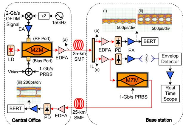
Fig. 2. Experimental setup for the proposed RoF system. Inset (i) The eye diagram of DL BPSK signal. (ii) The eye diagram of DL OOK signal. (iii) The eye diagram of UL OOK signal.
