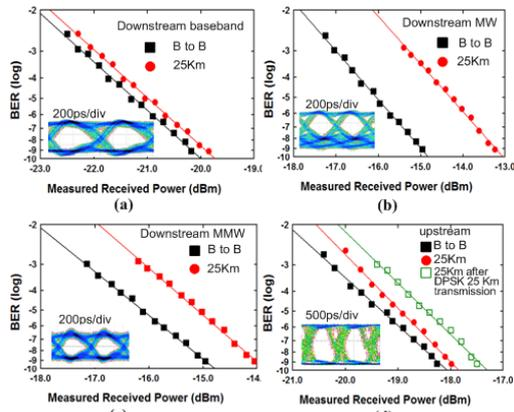
Fig. 2 BER performance and electrical eye diagrams
