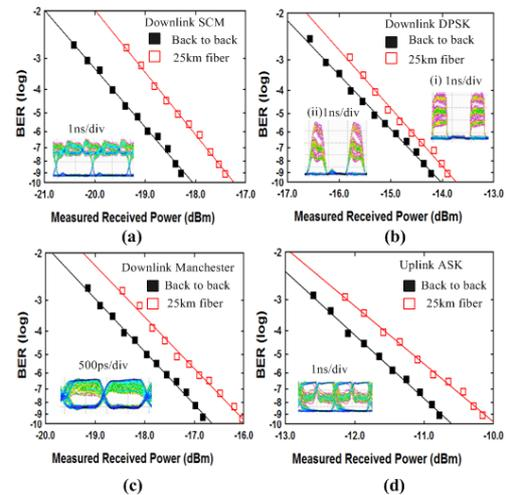
Fig. 4 BER performance and electrical eye diagrams
