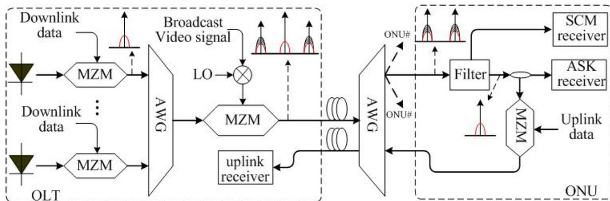
Fig. 1. Schematic diagram of the proposed WDM-PON system
