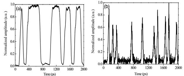
Fig. 5 a) and b) are waveforms of the input NRZ signal and the converted AMI signal, respectively.
