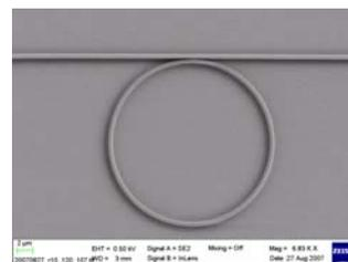
Fig. 1. SEM photo of a 10- $\mu\text{m}$  silicon microring.
