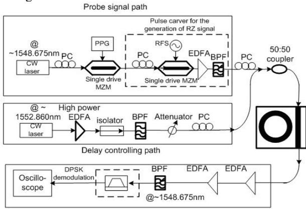
Fig. 2. All-optical tunable delay using a silicon microring.
