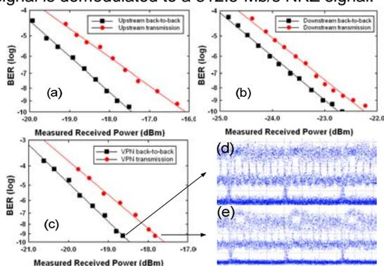
Fig. 3 BER measurements for the upstream transmission (a), downstream transmission (b), and VPN transmission (c); eye diagram of the reflected partial FSK signal before transmission (d), and after transmission (e).
