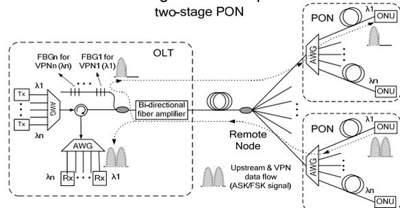
Fig. 1 The optical VPN in a two-stage PON.
