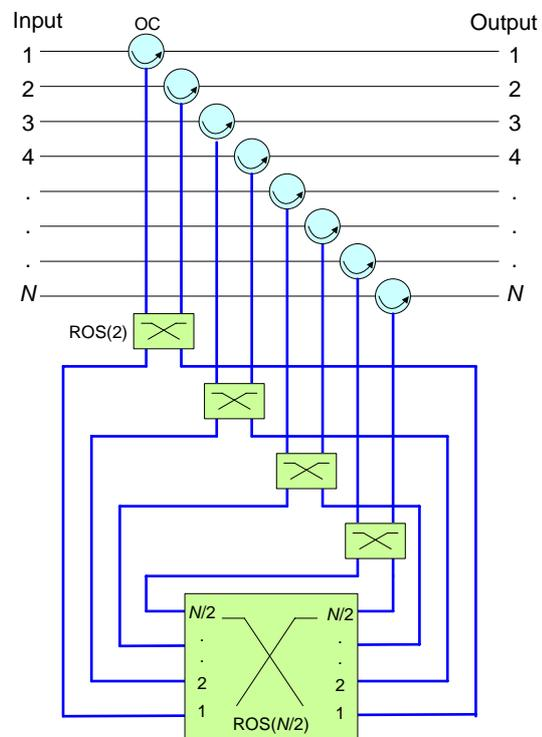
Fig.2 The architecture of proposed generic  $N \times N$  BOXC architecture. OC: optical circulator; ROS: reversible optical switch.
