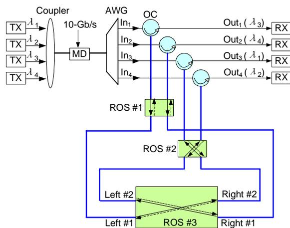
Fig.2. Experimental setup of the proposed BOXC prototype. OC: optical circulator; ROS: reversible optical switch. AWG: arrayed waveguide grating.
