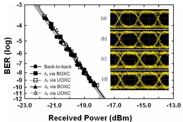
Fig.3. Measured BERs and eye diagrams. (a)  $\lambda_3$  via BOXC, (b)  $\lambda_3$  via UOXC (c)  $\lambda_4$  via BOXC and (d)  $\lambda_4$  via UOXC.
