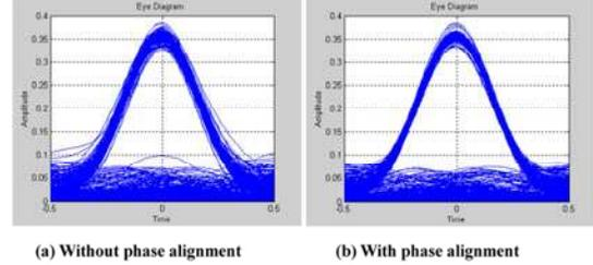
Fig.4 Eye diagrams of GAP(5)-CSRZ signal after transmission of 40 km SMF fiber (a) without phase alignment (b) with phase alignment.
