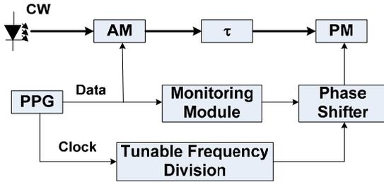
Fig.3 Schematic of data-pattern-assisted phase modulator
