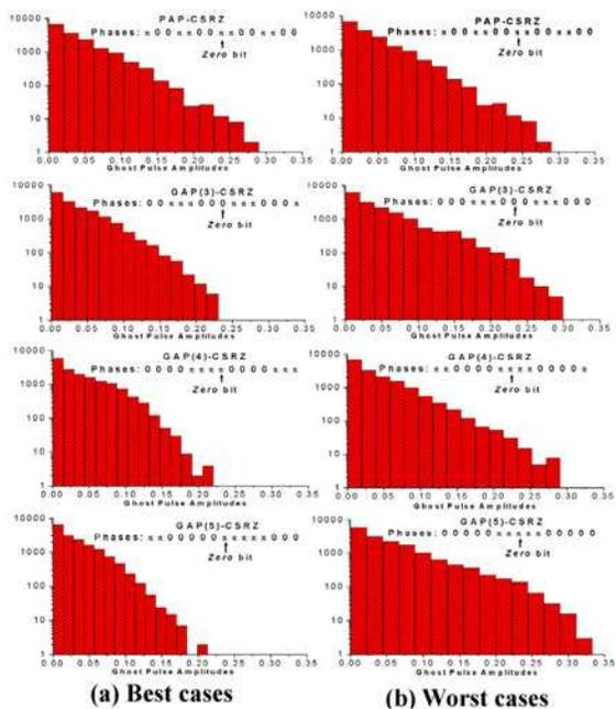
Fig.2 Histograms of ghost-pulse amplitudes for four formats with  $2^{14}$  possible bit combinations. (a) Best cases (b) Worst Cases.
