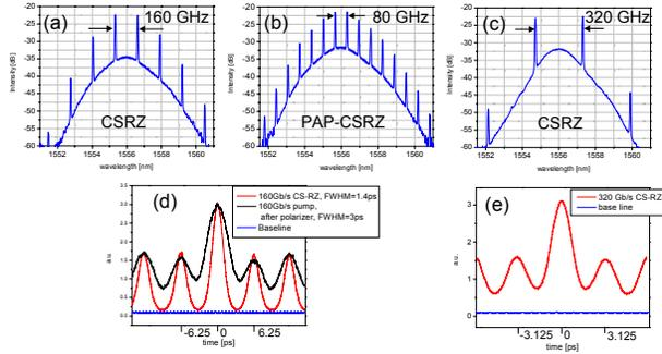
Fig. 4: spectra of a) 160-Gb/s CSRZ, b) 160-Gb/s PAP-CSRZ, c) 320-Gb/s CSRZ, and autocorrelation traces of d) 160-Gb/s and e) 320-Gb/s signals.
