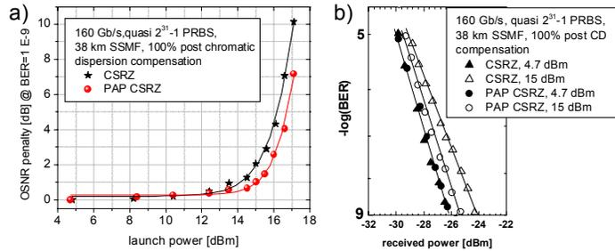
Fig.5: a) Sensitivity penalty due to NL propagation vs. launch power in SMF, b) BER curves for both formats at launch powers of 4.7 and 15 dm in SMF.
