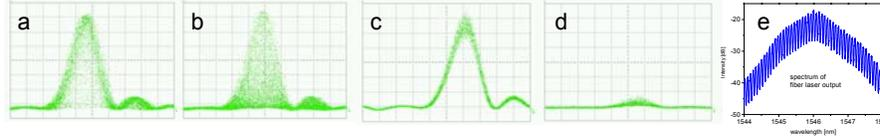
Fig.2: a) and b) interfered pulses from the fiber laser at the MZI constructive and destructive ports, respectively, c) and d) are the corresponding pulse waveform for the converted probe signal (5ps/div). and e) pump signal spectrum (0.01nm res.).
