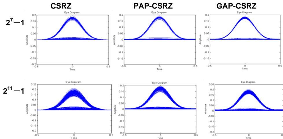
Fig. 3: Eye diagrams of the three signals with different pattern lengths after transmission through 30-km SMF fiber with a launch power of 15 dBm.
