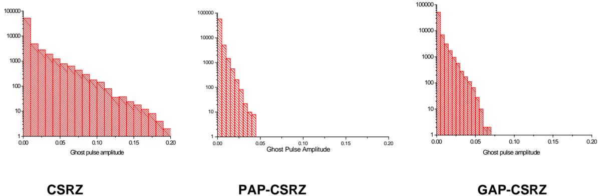
Fig. 2: Histograms of ghost pulse amplitudes for the three formats.
